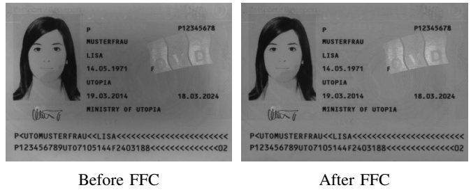
Fig. 6: Unprocessed vs. FFC-corrected IR sample of specimen passport illustrating the positive effect of FFC (for reader I).
